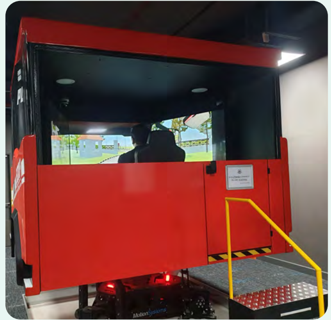
▲ Purpose-built driving simulator at the Civil Defence Academy to enhance driving training.
